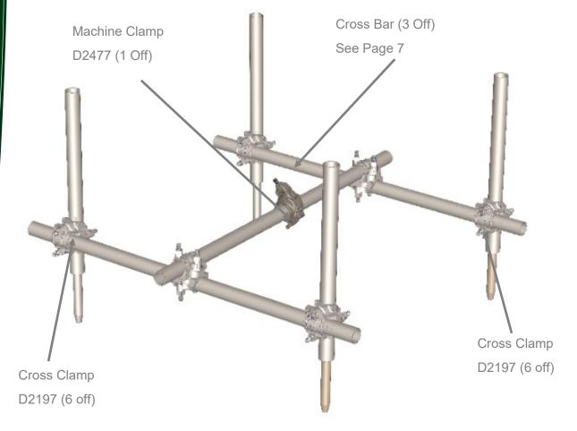
Note: this assembly is not available as a single part. This assembly must be ordered as a set of component parts.
