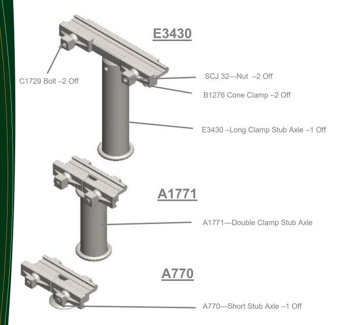
The long clamp stub axle is used in conjunction with the S36IR (independent rotation) drifter mounted on the Mk5 tandem motor screw feed shell and the short clamp stub axle is used in conjunction with the S36RB (Rifle bar rotation) drifter mounted on a Mk5 single motor feed shell.
