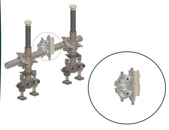
Close up detail of the short clamp stub axle locked in a cross clamp which is mounted on the horizontal bar of an H frame assembly. The stub axle can be easily rotated and set at any angle for accurate fan hole drilling where the axis of rotation has to be in line with the axis of the drifter. See page 9 for further details.
